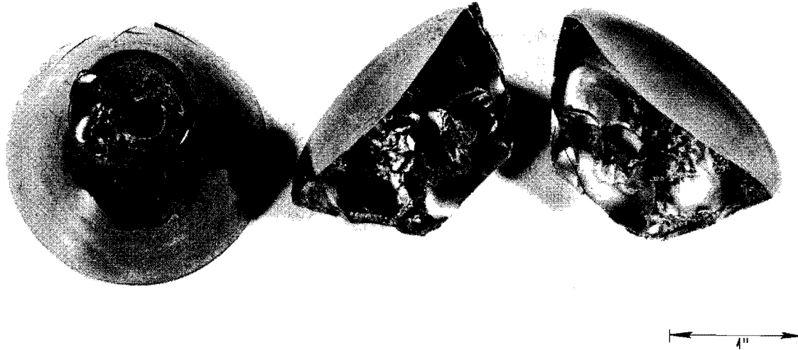
Fig. 5. Purex waste oxides were incorporated in phosphate-borate "glass." Waste made 1.5 M in H_3PO_3 , 0.8 M in MgO , 0.17 M in Na_2B_4O_7 , and 1.7 M NaOH , evaporated to dryness, and heated to 850^\circ C . Density 2.7 g/ml; product contained 39 wt % waste oxides; volume reduction factor, 5.5.
