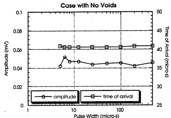
Figure 7 Amplitude of the first wave at the receiver and wave transit time between the transmitter and the receiver as a function of pulse width
