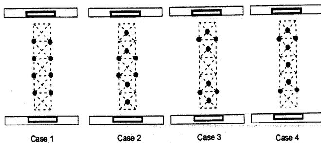
Figure 12 Various arrangement of eight stainless steel tubes
