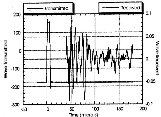
Figure 6 Typical transient data Measured for waves transmitted and received
