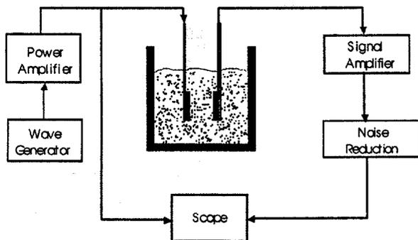
Figure 4 Block diagram of electronic apparatus
