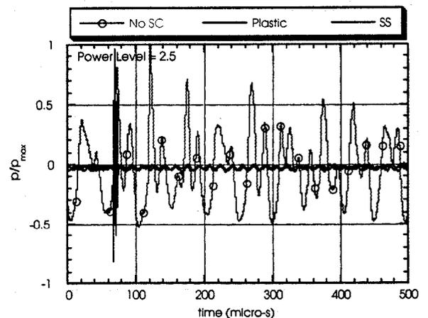
Figure 2 Wave forms with and without SCs in mercury
