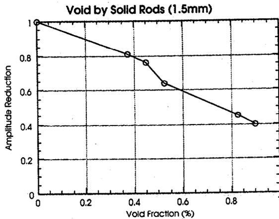
Figure 11 Wave attenuation in mercury as a function of void fractions (Solid Steel Rods)
