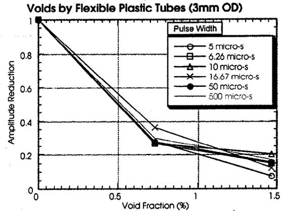
Figure 10 Wave attenuation in mercury as a function of void fractions (Plastic)
