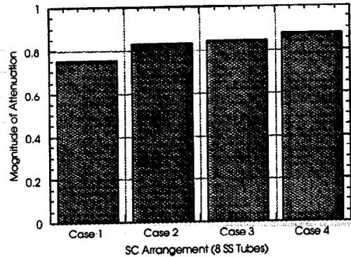
Figure 13 Wave attenuation for various arrangement of stainless steel tubes
