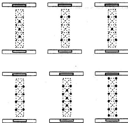
Figure 8 Arrangement of stainless steel tubes representing voids in mercury
