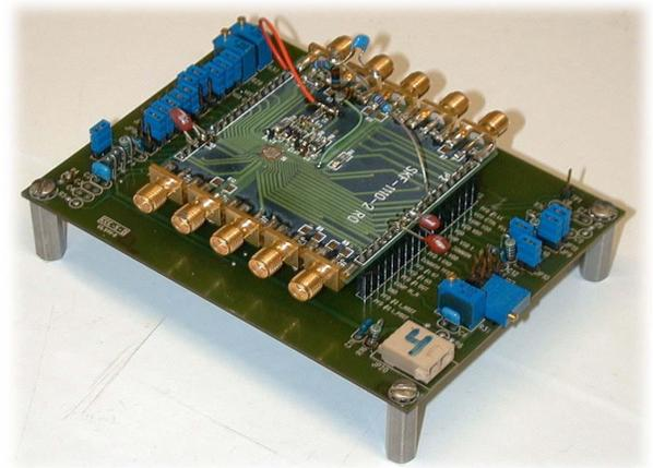
Figure 6. PLL test board.
