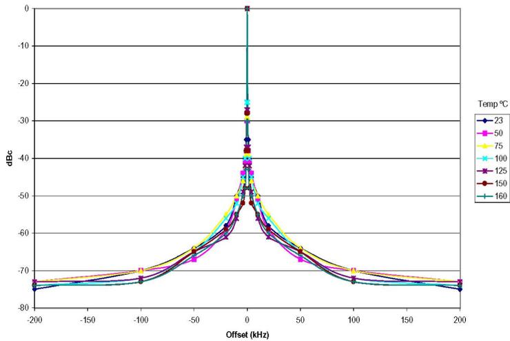
Figure 5. PLL Phase noise vs. Temperature.
