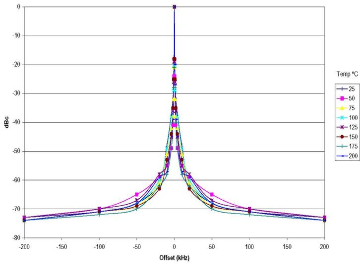
Figure 3. Open -loop phase noise of the VCO.
