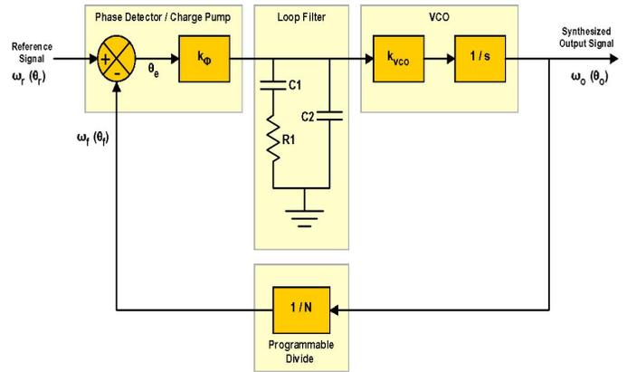
Figure 4. Block diagram of the PLL.
