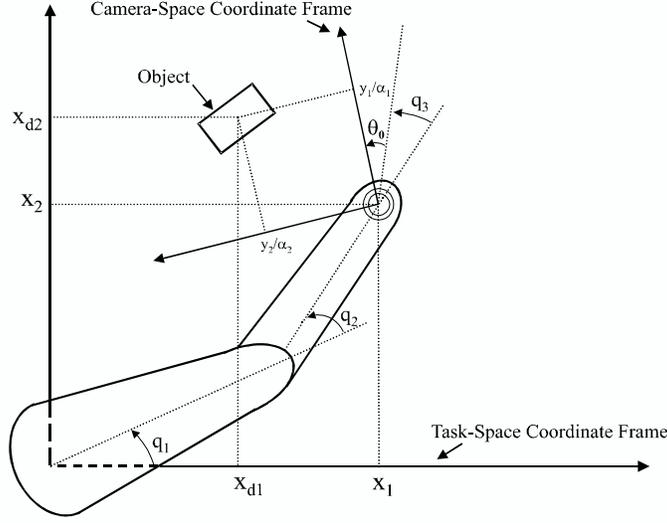
Figure 1: Three Link Robot Manipulator
