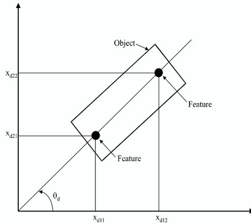
Figure 5: Geometric Relationship Between the Position of Object Features and the Object Orientation in the Task-Space
