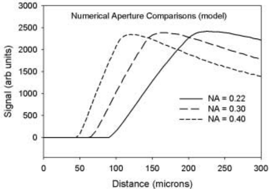
Figure 8: Comparison of model results for differing numerical aperture.
