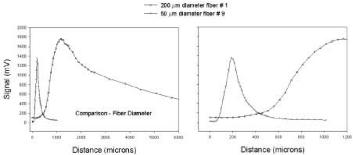
Figure 9: Comparison of 50 and 200 micron diameter fibers.
