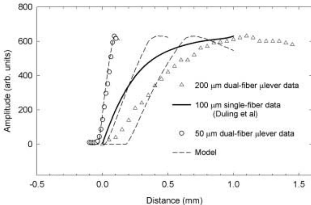
Figure 10: Comparison data for 50, 100 (single fiber), and 200 micron fiber.
