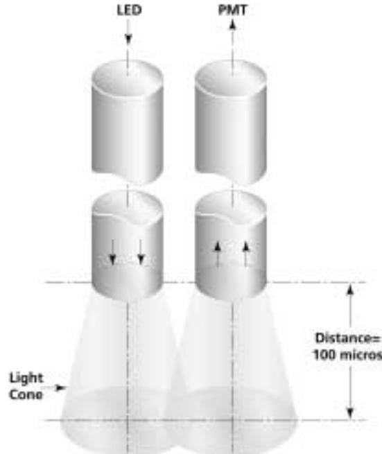
Figure 1: Dual-fiber reflective probe.
