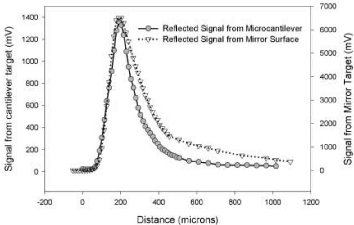
Figure 4: Comparison of Microcantilever and Mirror Signal vs Distance.
