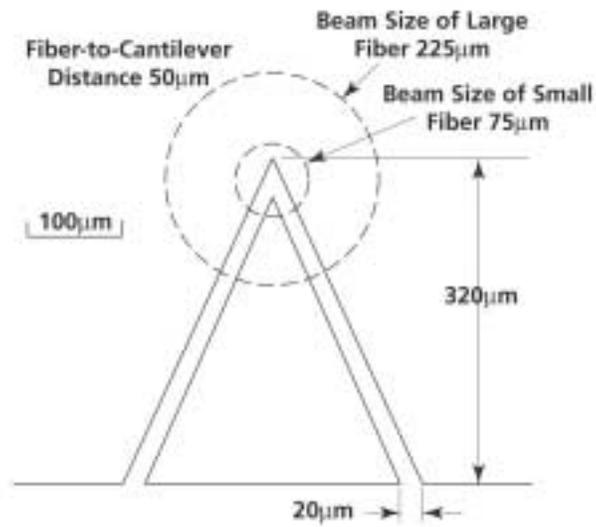
Figure 2: Microcantilever in relation to beam profiles.
