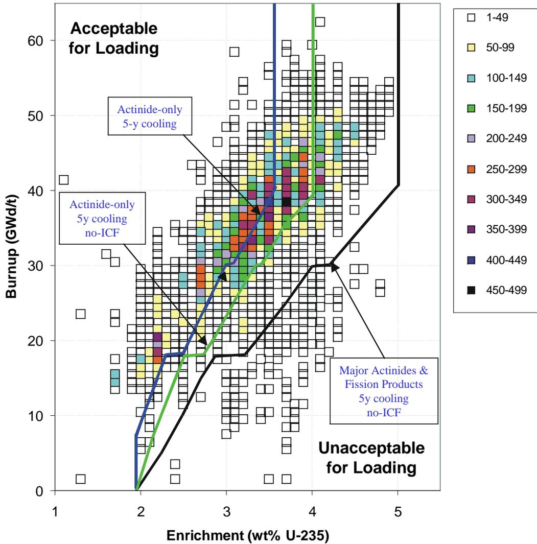
Figure 3. Illustrative loading curves for GBC-32 cask with 17×17 fuel assemblies calculated using the search capability in STARBUCS, plotted over the inventory of discharged PWR fuel up to 1999 (numbers in legend indicate the number of assemblies).
