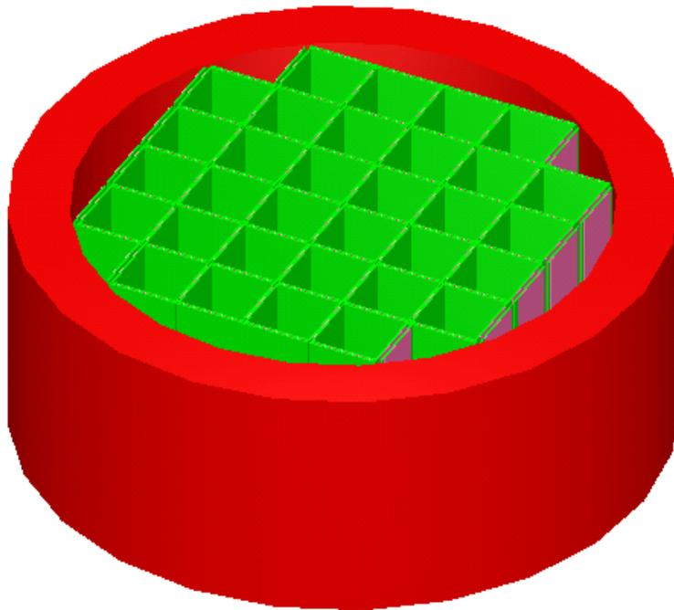
Figure 2. Cross-section view of the GBC-32 cask (unloaded)
