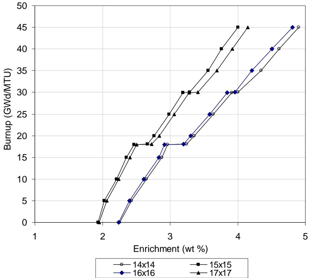
Figure 4. Illustrative loading curve for actinide-only burnup credit nuclides in 14×14, 15×15, 16×16, and 17×17 fuel assemblies in the GBC-32 cask, calculated using the search capability in STARBUCS.
