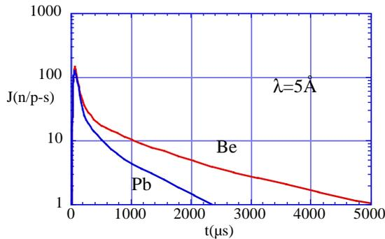
Fig. 7. Comparison:pulse from a H<sub>2</sub> moderator when a Be reflector is used and when a Pb reflector is used.
