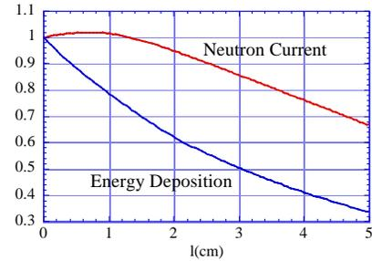
Fig. 13. Thermal neutron current and energy deposition vs the premoderator thickness( $l$ ).
