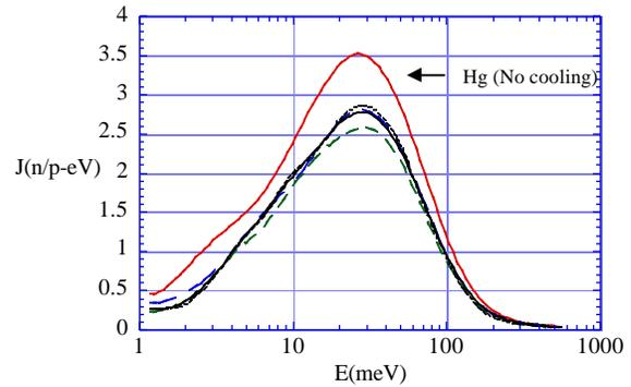
Figure 6. Neutron current from a H<sub>2</sub>O moderator for various target materials: Mercury with no cooling (solid), Mercury with D<sub>2</sub>O (long dashed), Tantalum with D<sub>2</sub>O (short dashed), and Tungsten with D<sub>2</sub>O (dotted).
