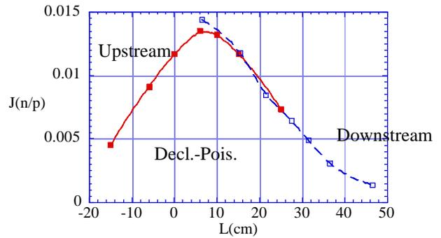
moderators are decoupled and poisoned the current is equal when they are at the same position.
