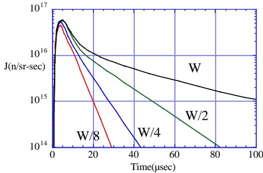
Figure 5. Neutron pulse ( $\lambda = 0.6$  to  $1.0 \text{ \AA}$ ) for various locations of a gadolinium poison plate. The distance  $W$  is measured from the viewed moderator face (the width of the moderator is  $W$ ).
