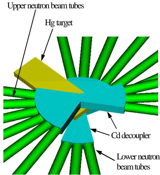
Figure 3. Full target station model with shielding and reflector assemblies removed.
