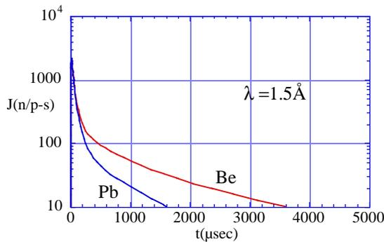
Fig. 8. Comparison:pulse from a H<sub>2</sub>O moderator when a Be reflector is used and when a Pb reflector is used.
