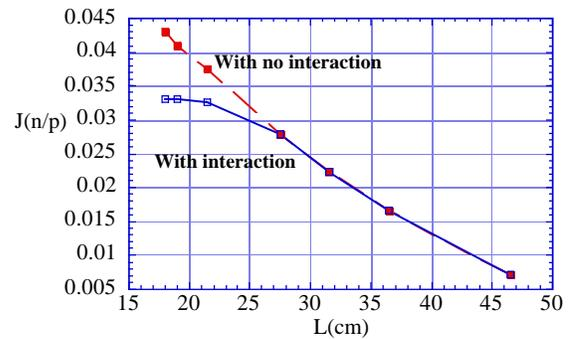
Fig. 11. Effect of moderator interaction on downstream coupled H<sub>2</sub> moderator output. Upstream moderator is a decoupled poisoned H<sub>2</sub>O moderator located at L=6cm.
