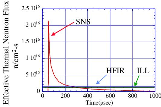
Figure 4. Expected performance of SNS compared to the HFIR and ILL reactors.
