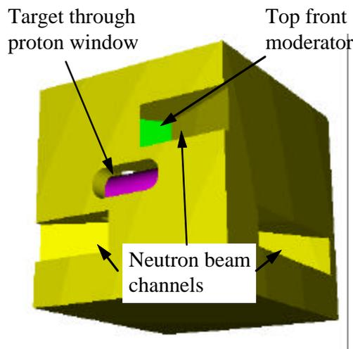
Figure 1. Outside of initial target station model.
