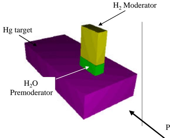
Fig. 12. Model geometry used for the premoderator study.
