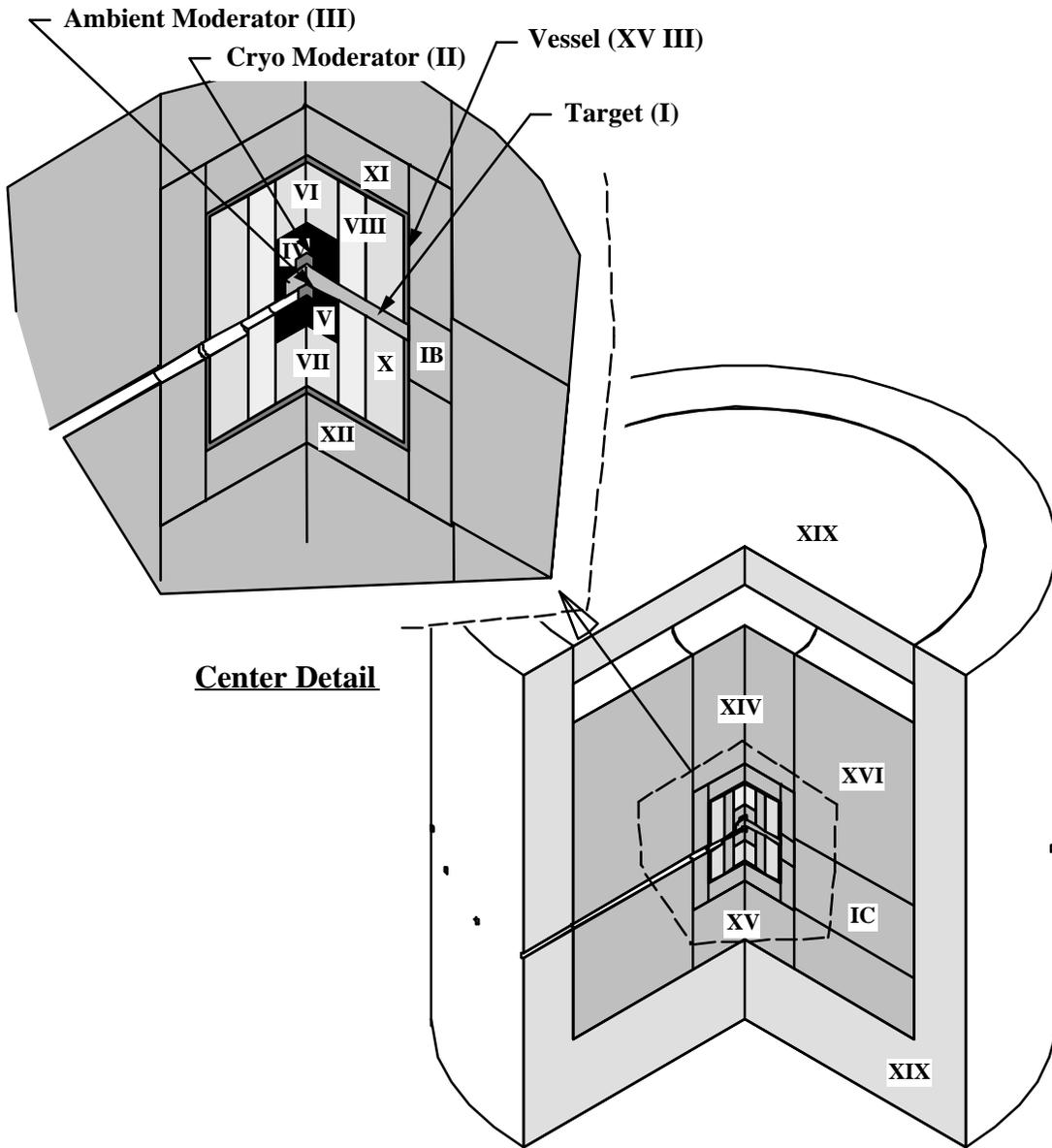
Figure 2. Schematic diagram of full target station model.
