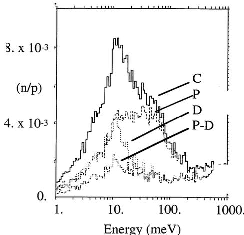
Fig. 6: Thermal neutron pulse from the face of the front front cryogenic moderator.
