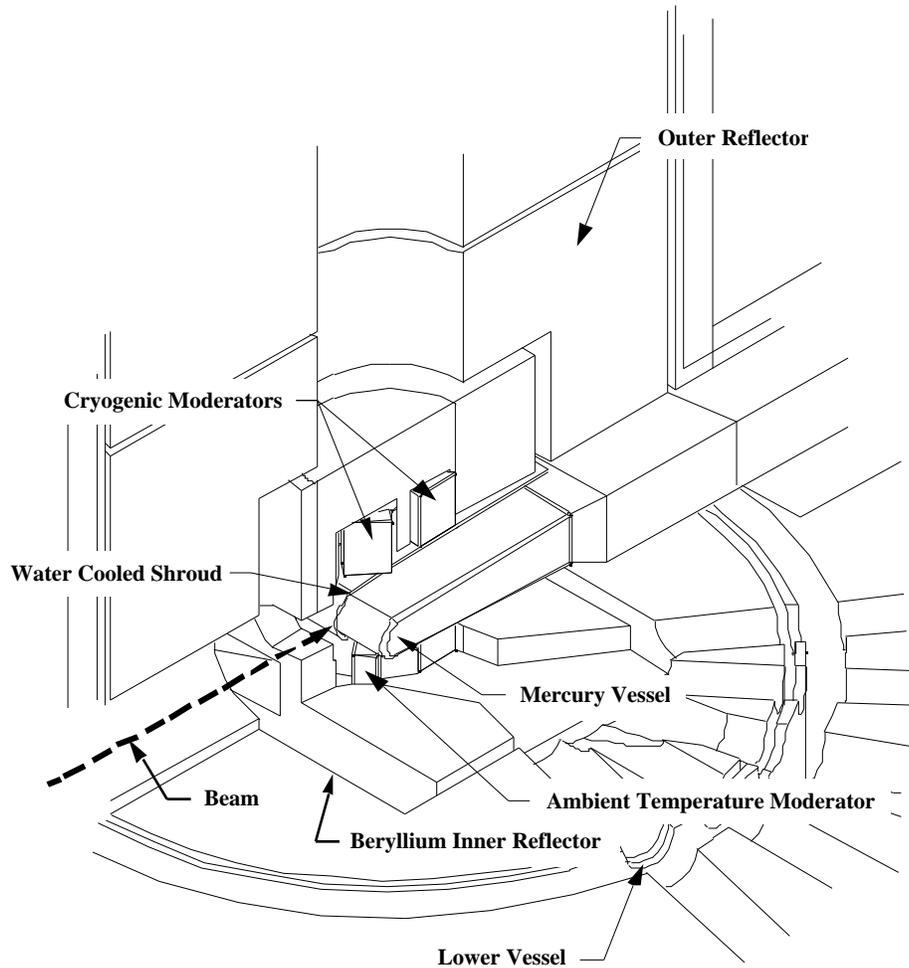
The heat deposited in the mercury target is transported away in the flowing mercury loop to a primary heat exchanger that is located on the target cart assembly, outside the target region shielding. The primary heat exchanger is a shell and tube type with mercury flowing in the tube side and the secondary coolant, i.e., demineralized water, flowing in the shell side. The tubes in this heat exchanger are a special, double-walled type which reduces the probability of a mercury leak into the
