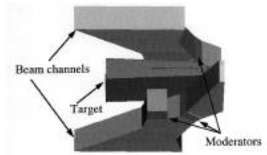
Figure 5. Neutronics models of overall target station
