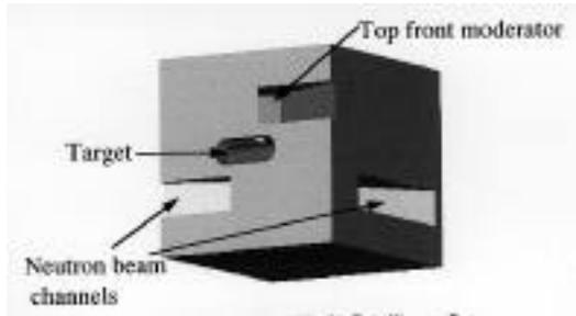
Figure 4b: Target, moderators, and the neutron beam channels as viewed from the bottom.
