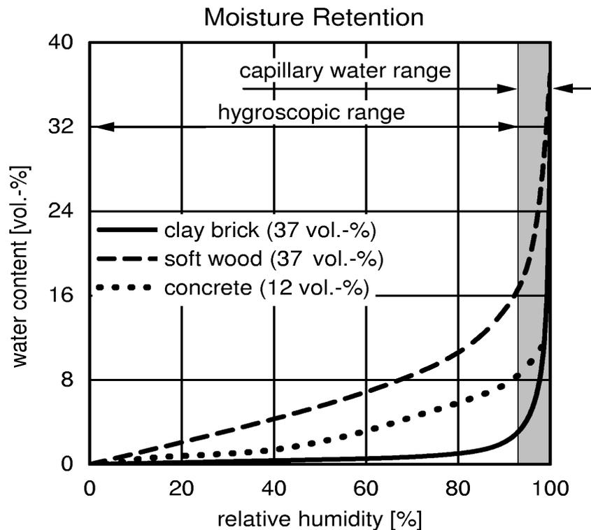
**Fig. 1:** Moisture retention curve for three typical building materials. The shaded area represents the part the capillary water range which is determined with pressure plate apparatus.
