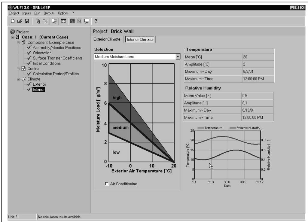
**Fig. 13: Enter Interior Climate Type (Low-Medium-High Load, or Air Condition)**
