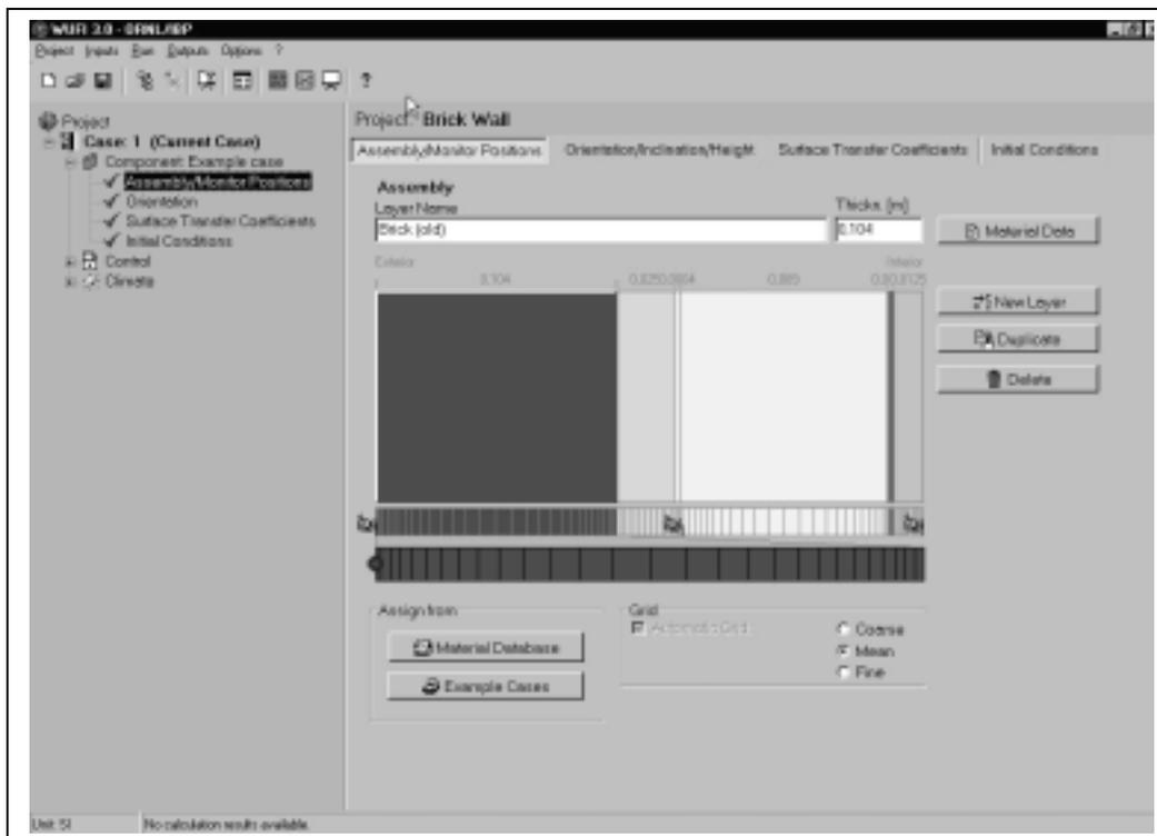
**Fig. 5: Enter Envelope Detail (dimensions, layout and monitors)**
