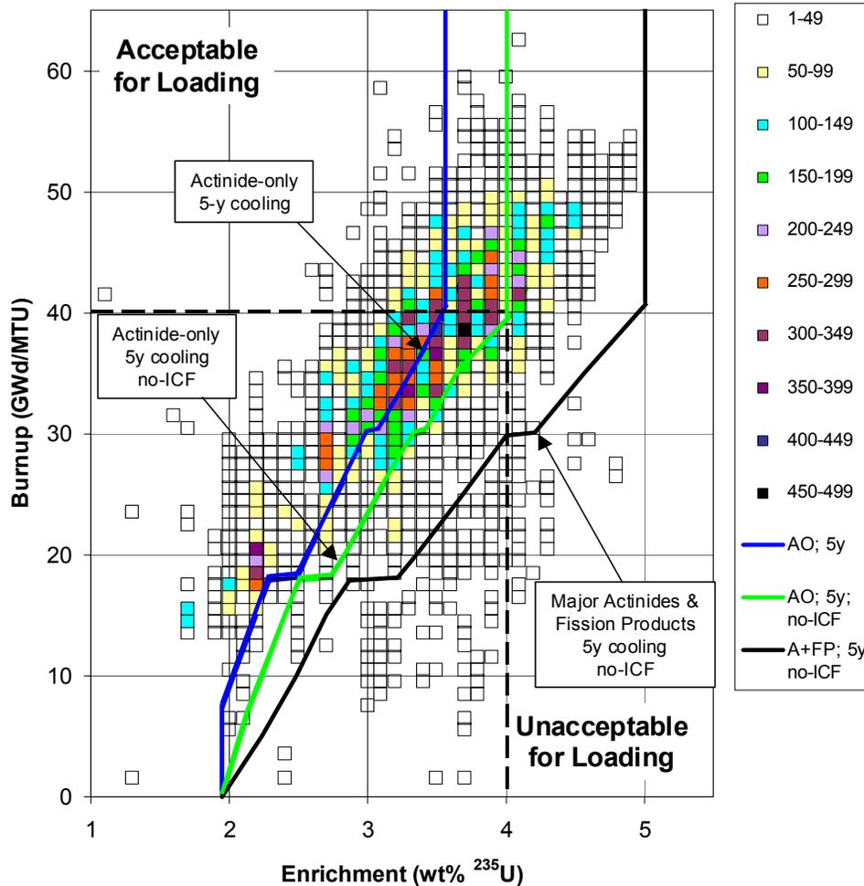
Figure 3. Illustrative loading curves for GBC-32 cask shown with PWR SNF discharge data through 1998 (numbers in legend indicate number of assemblies). Dashed lines represent current burnup and enrichment limits of ISG8.
