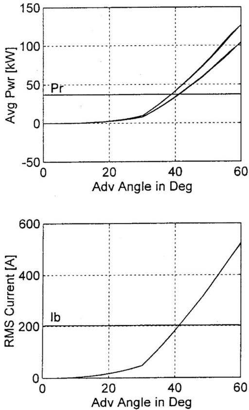
**Fig. 6. Average power and current vs advance angle at 7800 and 15600 rpm for  $V_{dc} = 183.4$  ( $n = 3$  and  $n = 6$ ) and  $V_{dc} = 150$  ( $n = 3.66$  and  $n = 7.32$ ) for  $L = 73.6 \mu H$ .**
