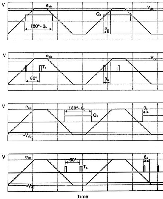
**Fig. 2. DMIC firing scheme for phase A semiconductors in the high-speed motoring mode.**
