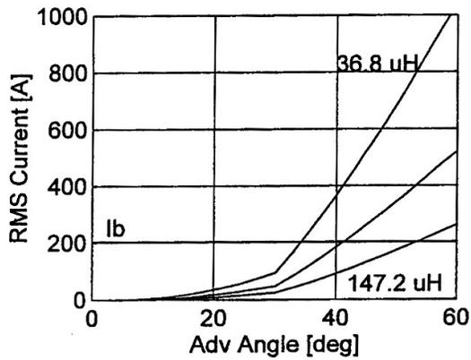
Fig. 8. Average power and rms current vs advance angle at 15600 rpm for motor inductances of 36.8 μH, 73.6 μH, and 147.2 μH.
