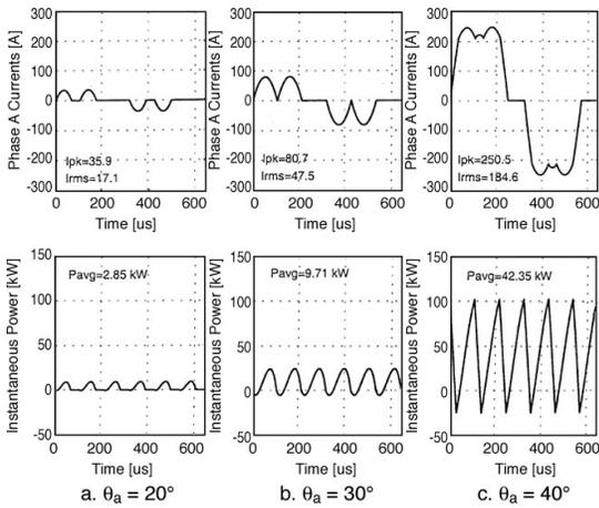
**Fig. 4. Instantaneous phase A motor current and power at 15,600 rpm ( $n = 6$ ) and  $V_{dc} = 183.4$  V.**
