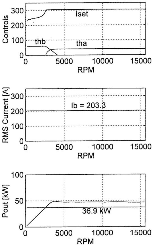
**Fig. 7. Performance envelope of DMIC with nominal motor parameters.**
