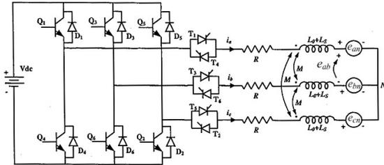
**Fig. 1. DMIC inverter topology and BDCM model.**
