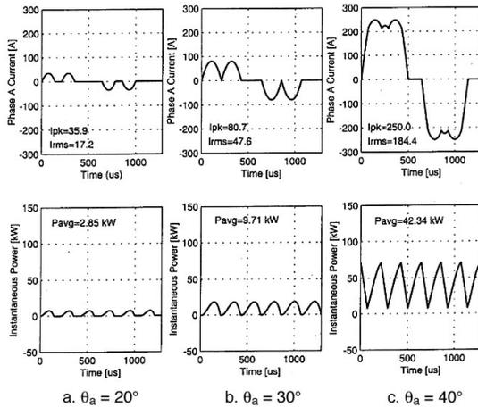
**Fig. 3. Instantaneous phase A motor current and instantaneous power at 7800 rpm ( $n = 3$ ) and  $V_{dc} = 183.4$  V.**
