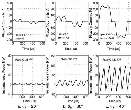
**Fig. 5. Instantaneous phase A motor current and power at 15,600 rpm ( $n = 7.32$ ) and  $V_{dc} = 150$  V.**
