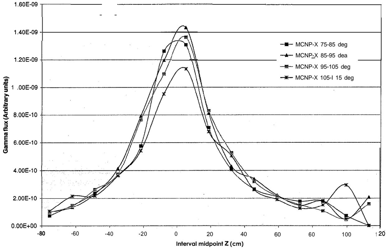
Fig. 6 Variation of gamma flux in the vertical direction at the outer surface of the shipping cask. Total gamma flux is shown for four azimuthal segments around the location of the maximum (at  $\sim 90$  degrees).
