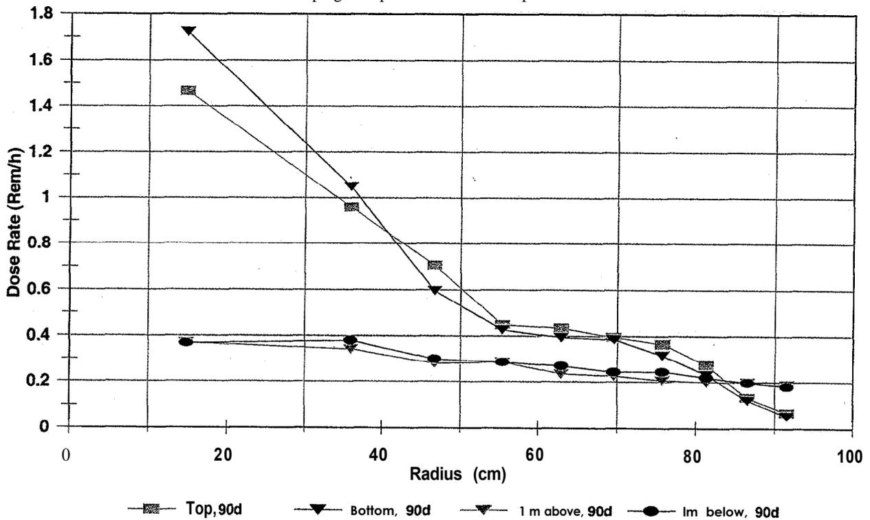
Fig. 8. Dose rate distributions at the shipping cask top lid, bottom lid, and at the distance of 1 m above the top and below the bottom.
