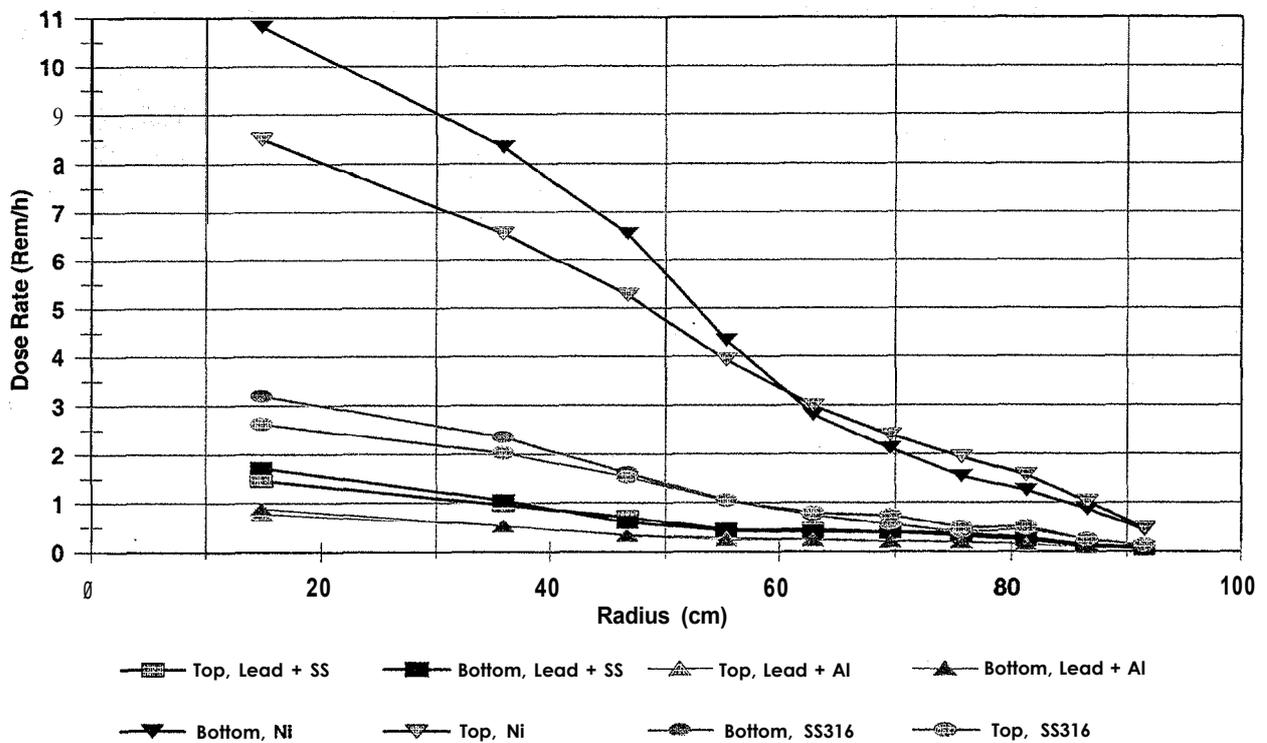
Fig. 10. Comparison of dose rates outside the cask lid and bottom for different inner plug material compositions.
