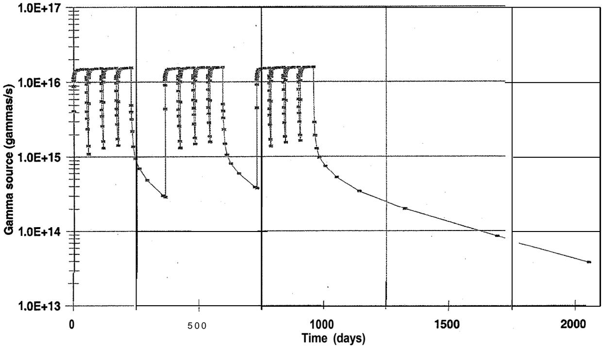
Fig. 5. Gamma source as a function of time for the lead-beryllium SNS inner plug.
