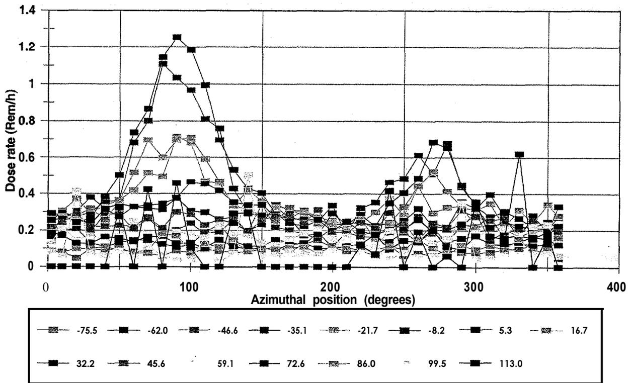
Fig. 7. Distribution of the dose rate on the outside surface of the shipping cask. Each curve corresponds to one axial segment, with the Z coordinate of the center of the segment given in the legend (in centimeters). The plug mid-plane is in the Z=0 plane.
