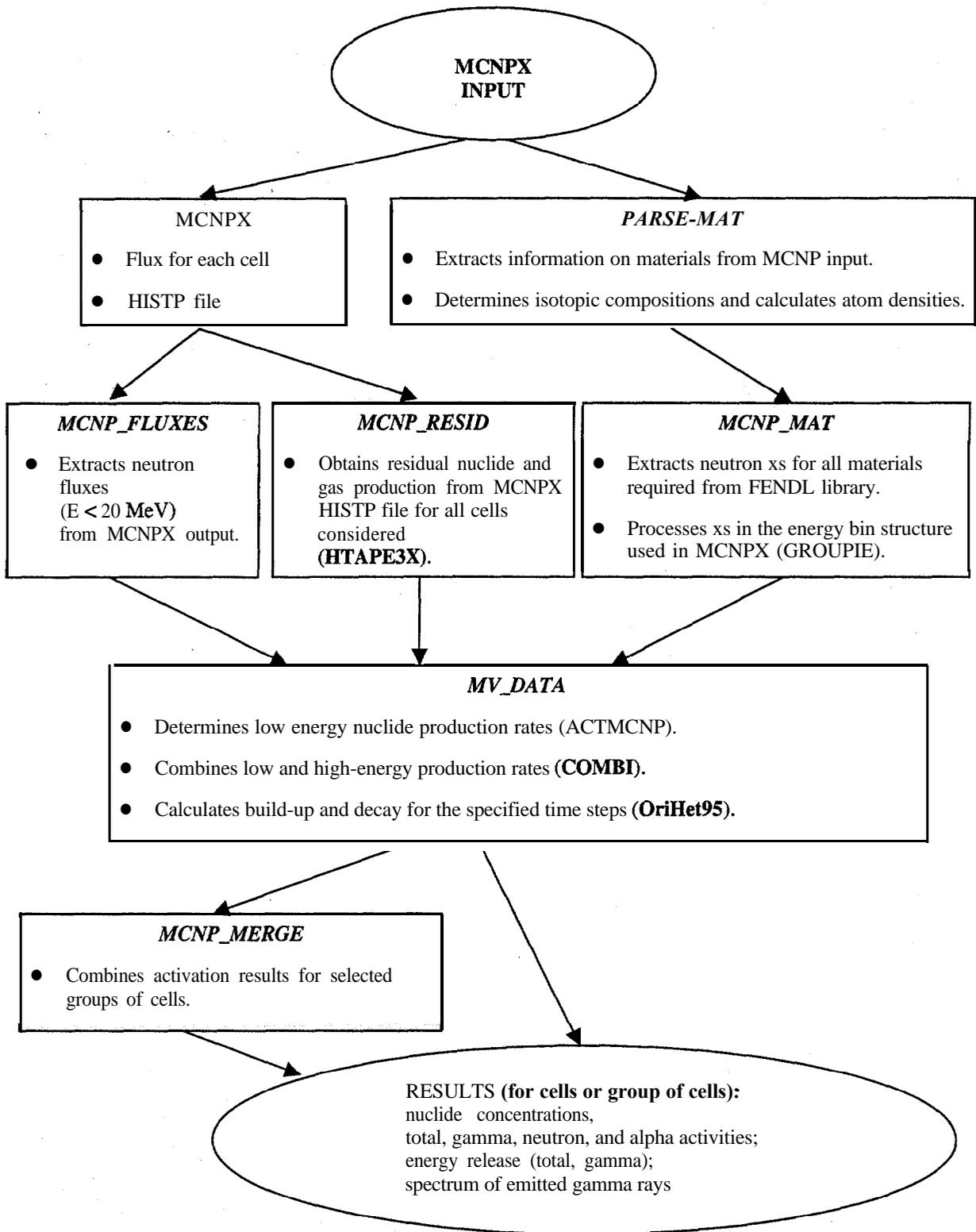
Fig. 4. The Activation Analysis System.
