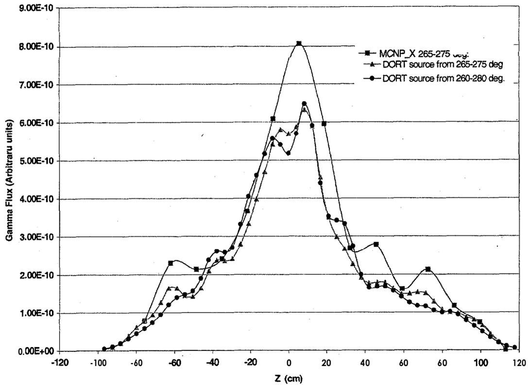
Fig. 9. Axial distribution of gamma fluxes obtained with MCNPX and DORT code.
