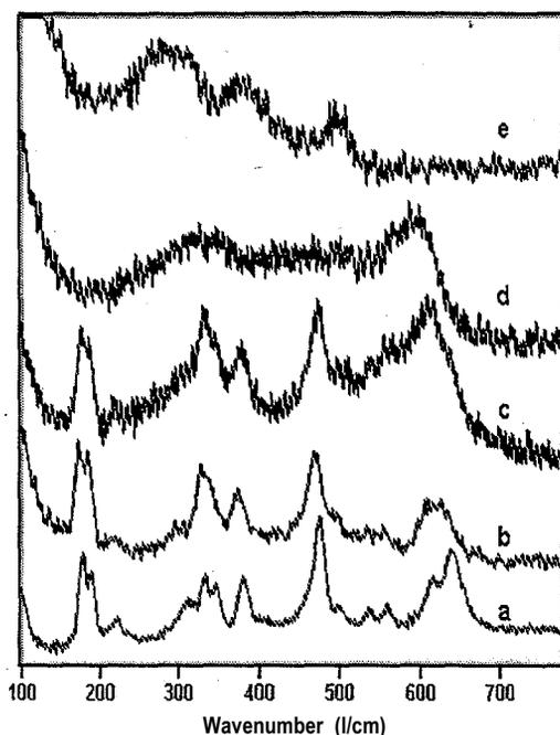
Fig. 2 Raman spectra of  $ZrO_2$ :Cm(III): a)  $m-ZrO_2$ ; b)  $Cm_{0.1}Zr_{0.9}O_{1.95}$ ; c)  $Cm_{0.2}Zr_{0.8}O_{1.9}$ ; d)  $Cm_{0.3}Zr_{0.7}O_{1.85}$ ; e)  $Cm_2Zr_2O_7$
