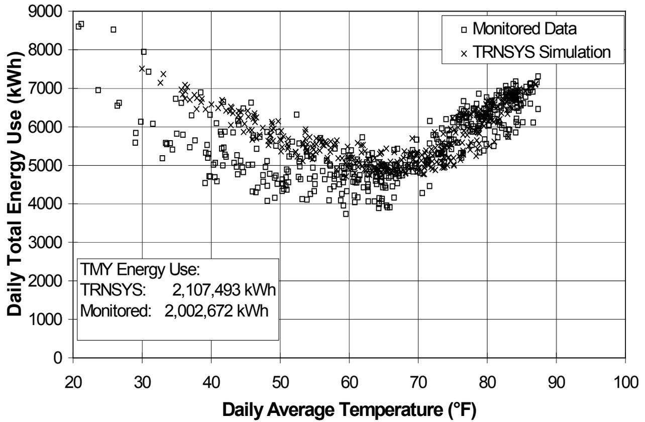
Figure 7: Total daily post-retrofit electrical energy use vs. daily average temperature for the Fort Polk Feeder, site-monitored and simulated by TRNSYS model.
