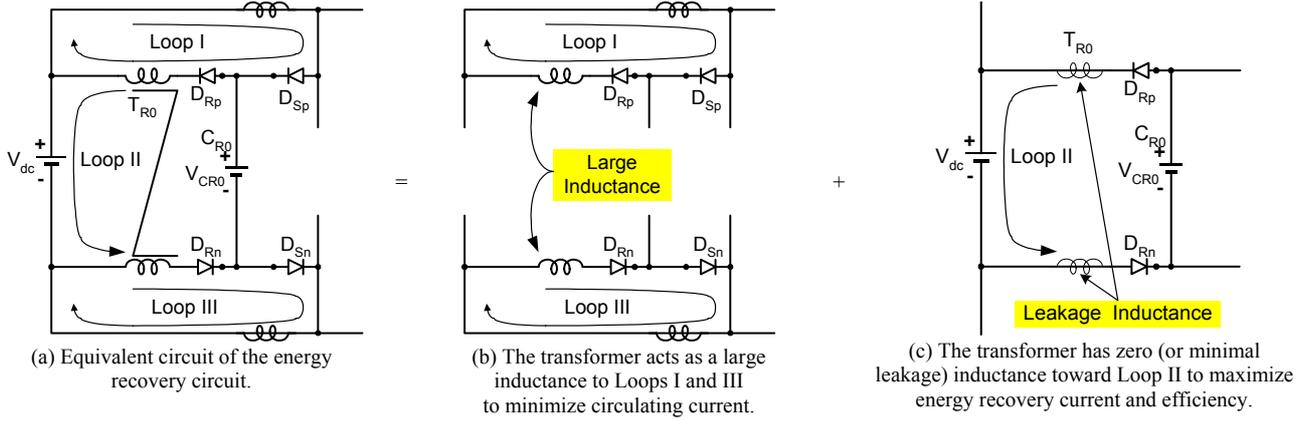
Fig. 5. Operating principle of the energy recovery circuit.
