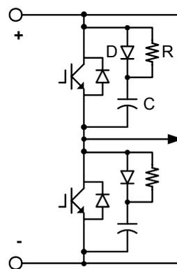
Fig. 1. An inverter phase leg with RCD snubbers.
