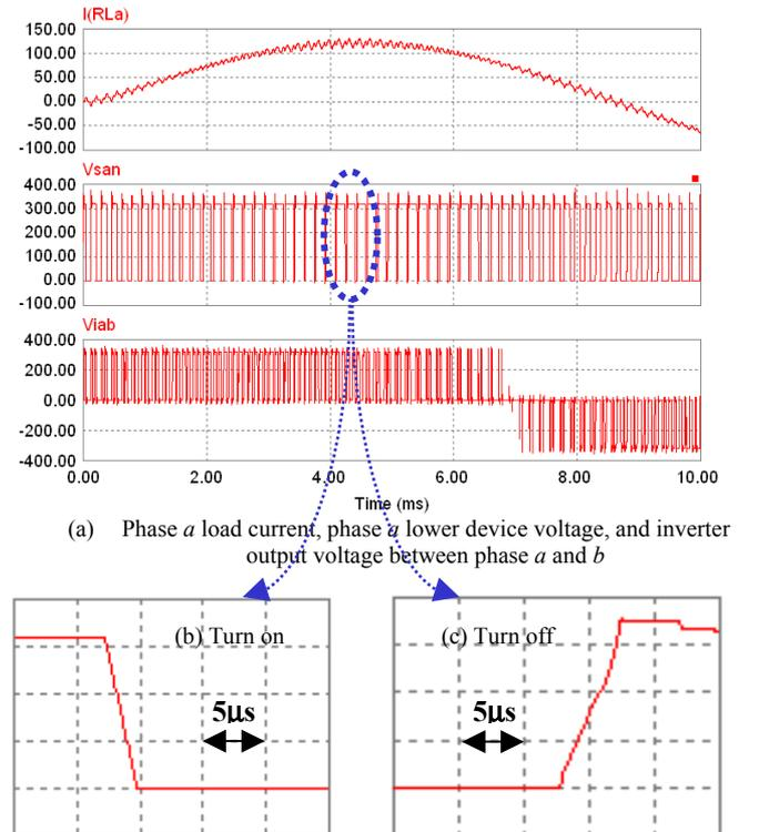
Fig. 6. Simulation waveforms.
