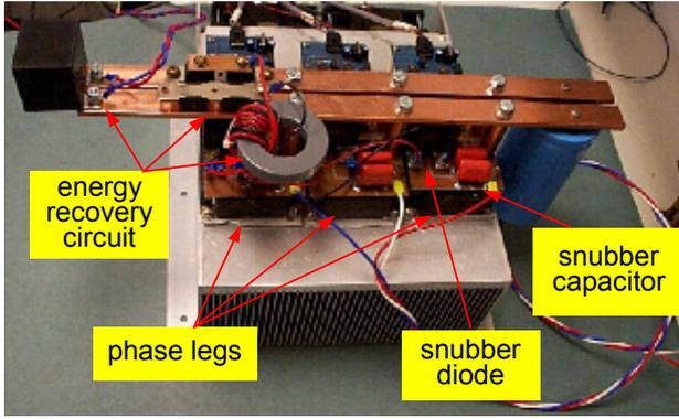
Fig. 7. Photo of a 150 kVA PSSS inverter prototype.
