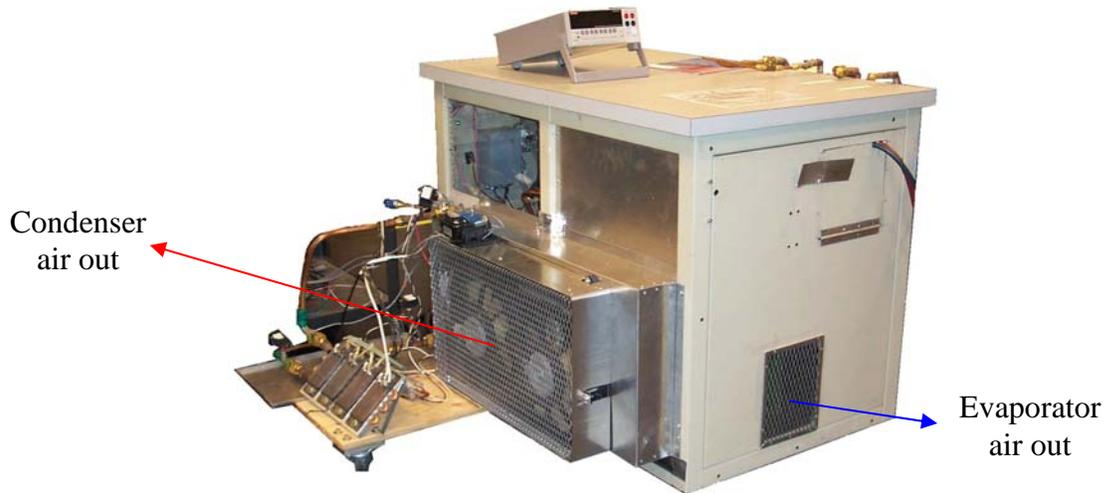
**Fig. 1. Floating loop attached to full sized sedan AC system in a cabinet.**
