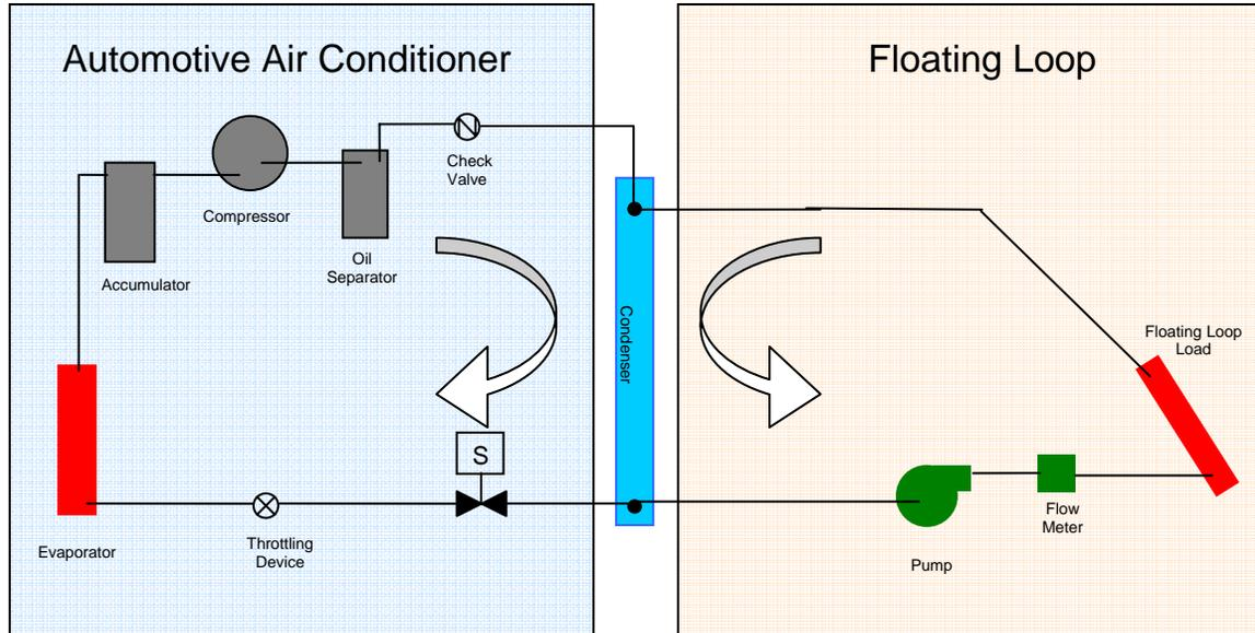
**Fig. 2. Floating loop/AC schematic.**
