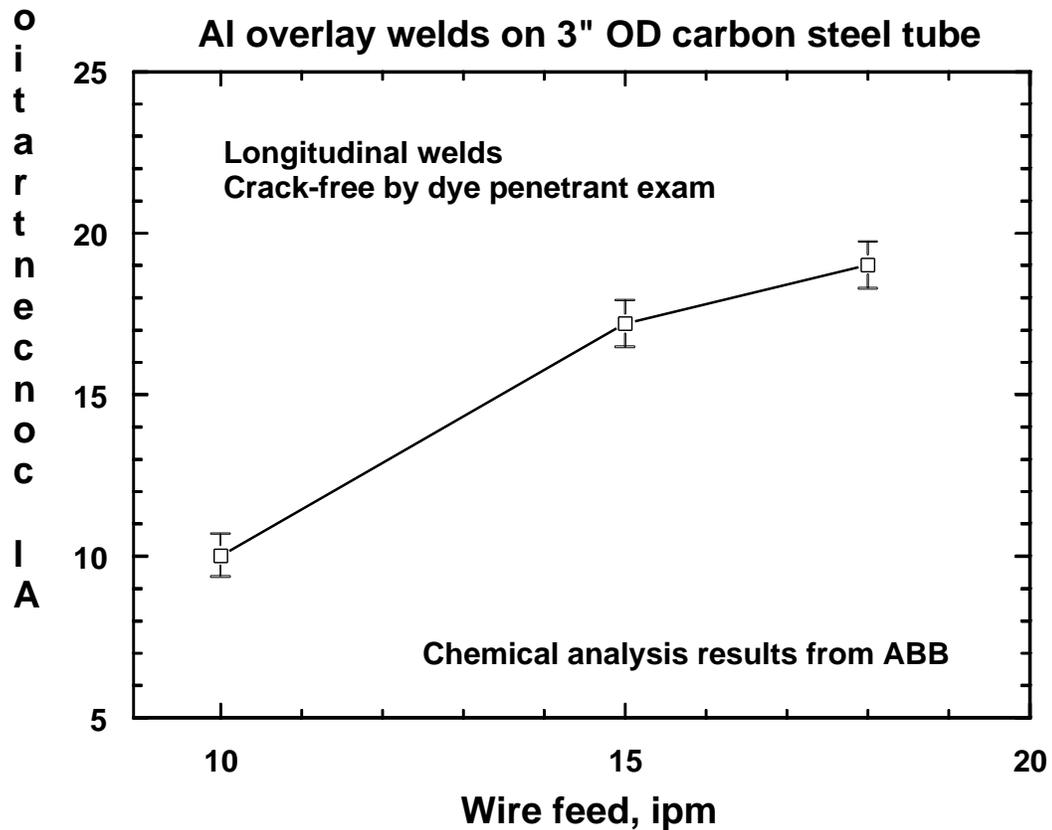
Fig. 4. Plot showing the variation of aluminum concentration in weld deposits on carbon steel with the rate of addition of aluminum wire into the weld puddle.
