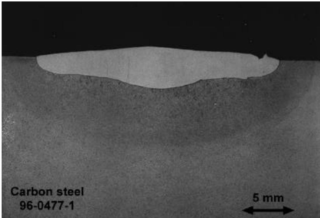
Fig. 2. Cross-sectional view of weld bead made by depositing aluminum wire on carbon steel using the gas-tungsten arc welding process.
