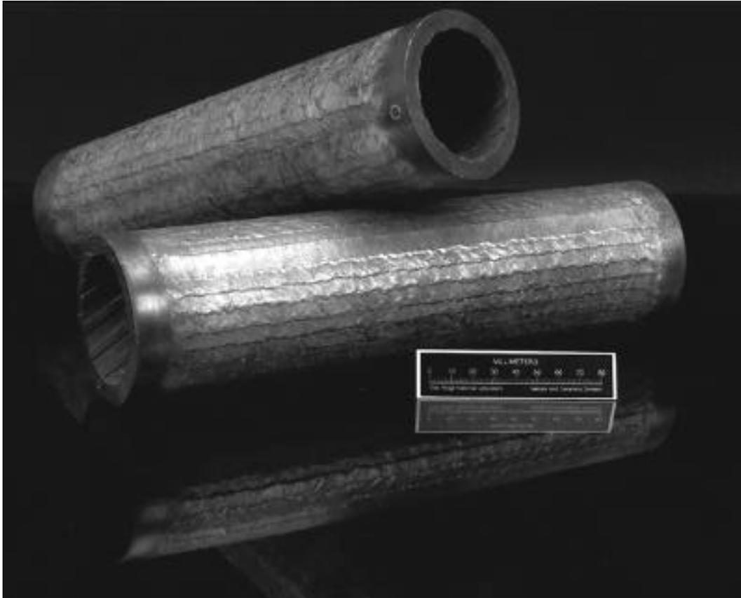
Fig. 3. Sections of 75-mm-diam carbon steel tubing that were aluminized by automatic gas-tungsten arc welding.
