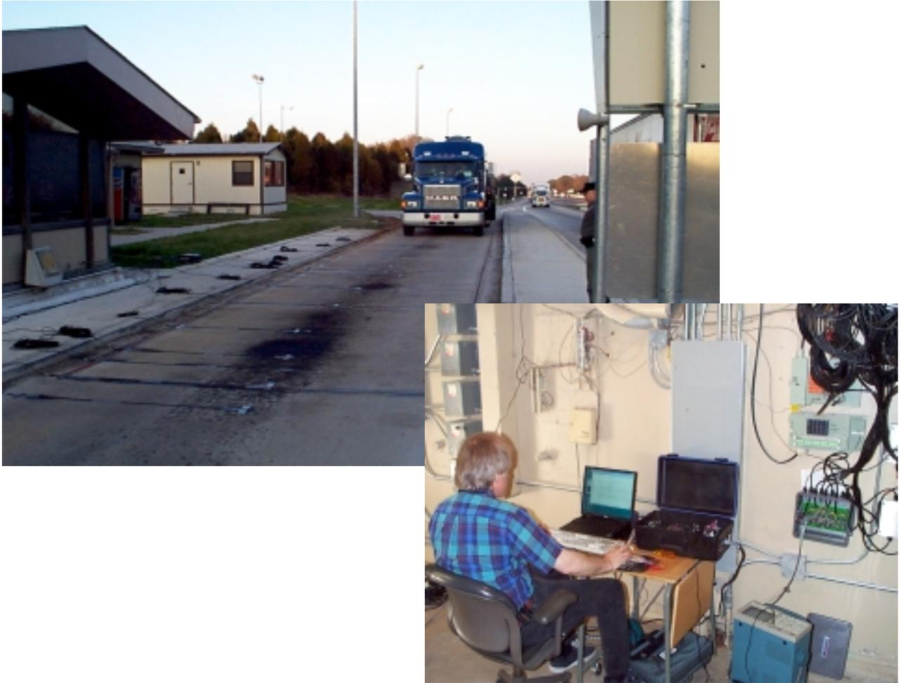
Figure 3 – Photo of SSC-WIM at I-40/75 Knox County Weigh Station
