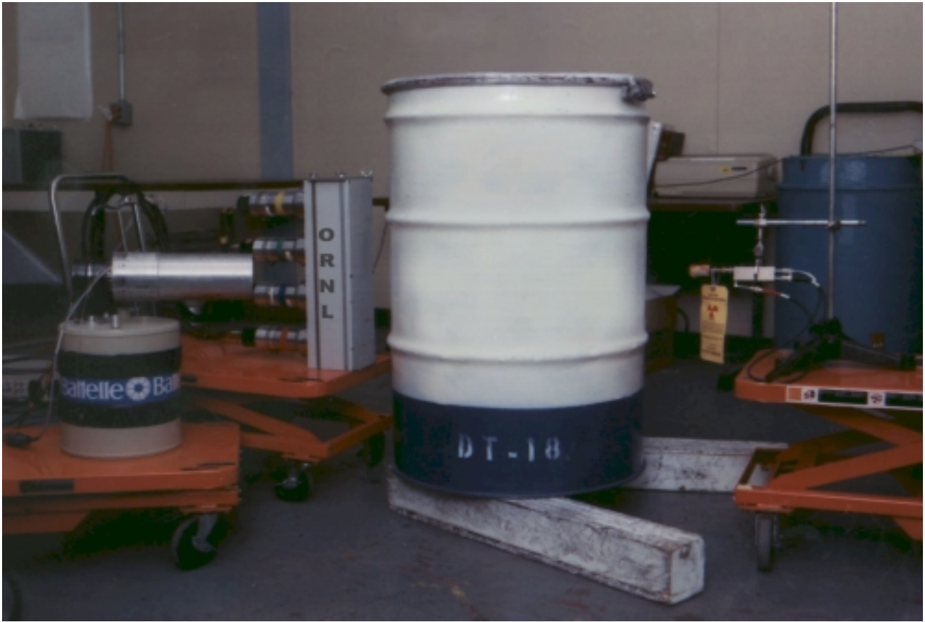
Fig. 2. Simultaneous NMIS-Gamma Ray Spectrometry Measurements For Fissile Material in a Container.
