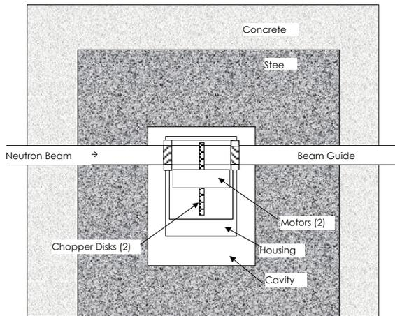
Figure 3. Schematic cross section of bandwidth chopper model showing principal components. Chopper is Cd-coated aluminum disk.
