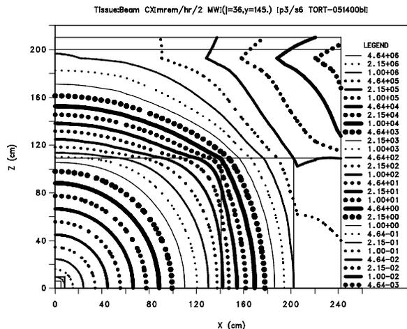
Figure 5. Vertical cut plane through beam line model, showing dose contours (mrem/h). Location is approximately at maximum. Lower and left edges are symmetry planes, floor is at top and side wall is to right.
