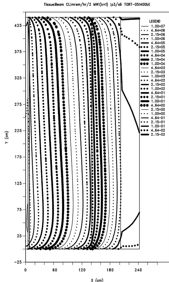
Figure 6. Tissue dose contours (mrem/h) on a horizontal plane through the beam line centerline. Left edge is the symmetry plane and center of the beam.
