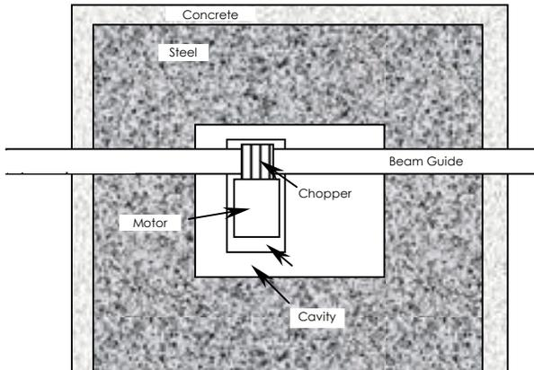
Figure 2. Schematic cross section of the  $E_0$  chopper model, showing principal components. The chopper is a laminate of boron and aluminum plates.
