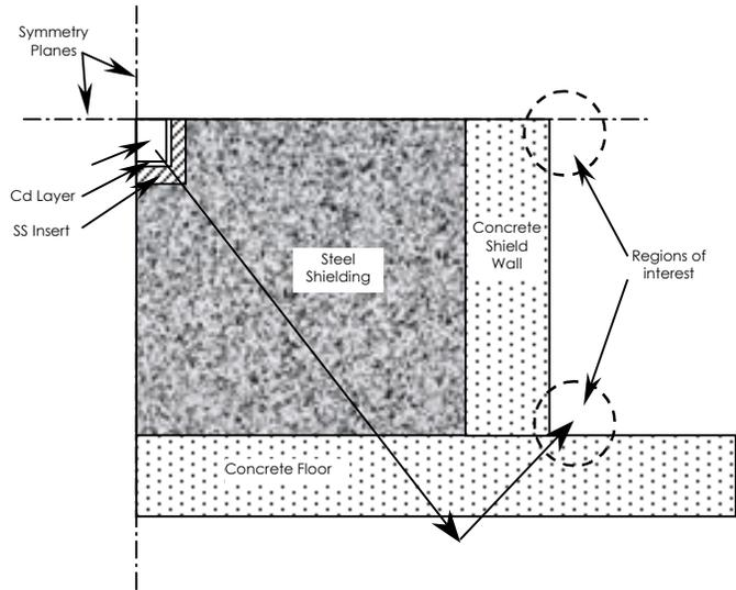
Figure 4. Schematic cross section of the TORT 3-d beam line model. The left-hand and upper boundaries are symmetry planes.
