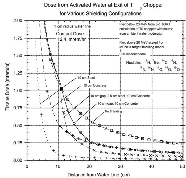
Figure 10 Tissue dose as a function of distance, from a  $T_0$  chopper water cooling line, with various shielding configurations.
