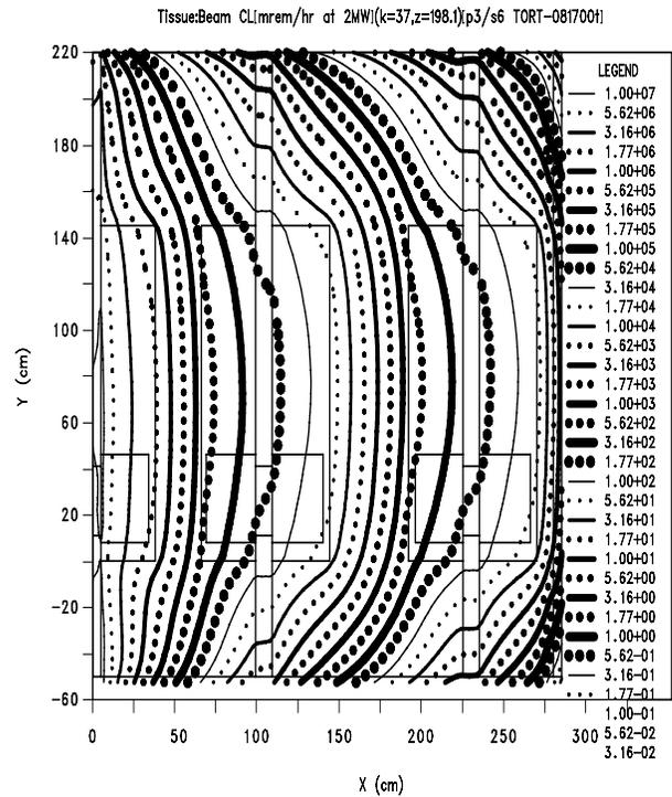
Figure 8. Dose contours (mrem/h) on a horizontal plane through the center of the 3-cavity T<sub>0</sub> chopper model.
