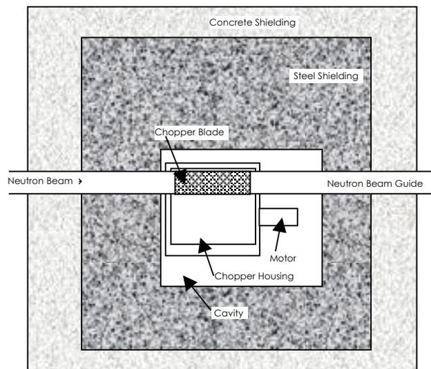
Figure 1. Vertical cross section of  $T_0$  chopper, showing typical chopper components included in the model.
