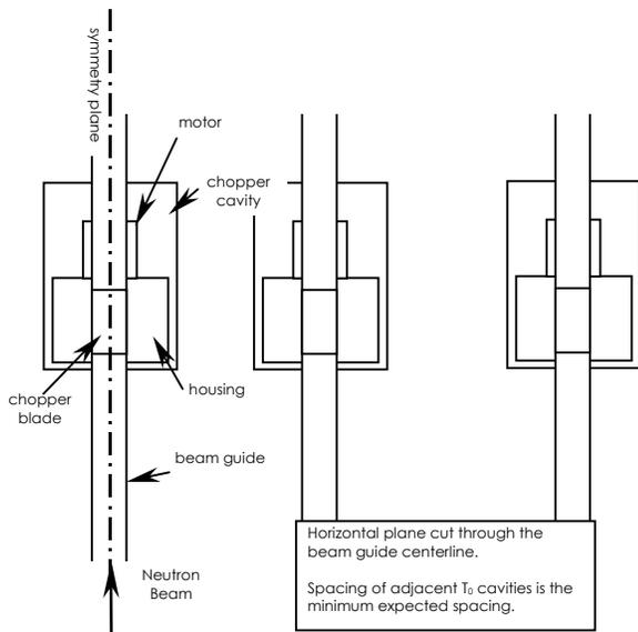
Figure 7. Schematic plan view diagram of 3-cavity T<sub>0</sub> chopper model. Left-most chopper is active. Symmetry boundary is on centerline of left chopper and beamline.
