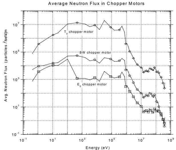
Figure 9 Neutron flux spectrum in the motors of each chopper type, at their respective “worst-case” locations.
