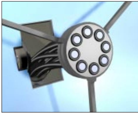
Figure 6b. Close-up view of large-core optical fiber ends.
