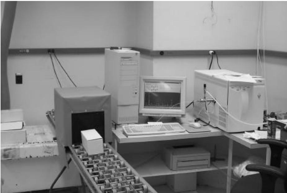
**Figure 9: A box enters the simulated chokepoint for DSITMS interrogation.**
